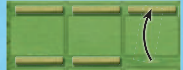
Gaining land by moving the Dike Line
